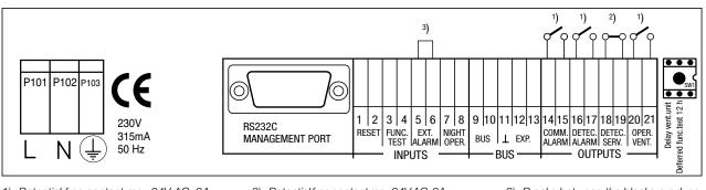
1) Potential free contact max 24V AC, 3A. Drawn in dead state/alarm mode. 2) Potential free contact max 24V AC, 3A. Drawn in dead state/normal mode.
