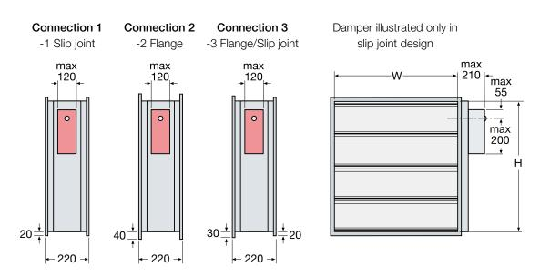
RABR for installation in combination with RBVG supplied with connection type 3 Slip joint/Flange. RABR 250, 450, 650 etc. in height is supplied with a raised slip joint or flange connection.
